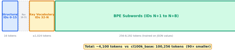
Figure 2: Three-tier vocabulary architecture. Token ID space is partitioned into structural tokens (blue), learned key vocabulary (gold), and BPE subwords (green). For a tokenizer with M = 46 learned keys and B = 4,096 BPE tokens, the total vocabulary is 32 + 46 + 4,096 = 4,174 compared to c1100k_base ’s 100,256.
